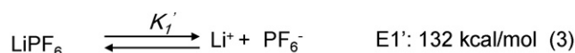
Fig. 2. The equilibrium equations for Li 2 DFB and LiPF 6 , energy difference between salt and dissociated state was calculated by MO method.
